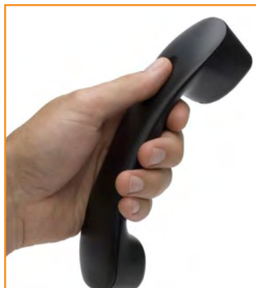
Figure 10: A user may hold a handset with a thumb on the back, using the finger notch.
